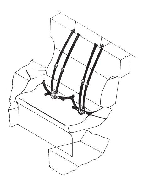
Figure 4-1. Seating Arrangement, Two-Passenger Operation
