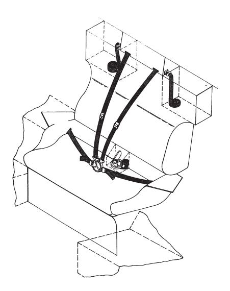
1. Use outboard seat belt and rotary with inboard shoulder harnesses for one-passenger operation. Stow unused harnesses in pockets above seat back. Stow unused seat belt and right hand rotary through slot in center of seat cushion.
