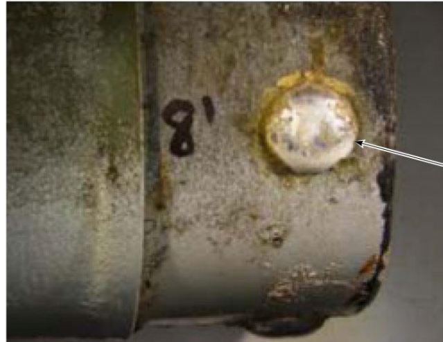
INCORRECT PLAIN "A" TYPE RIVET
