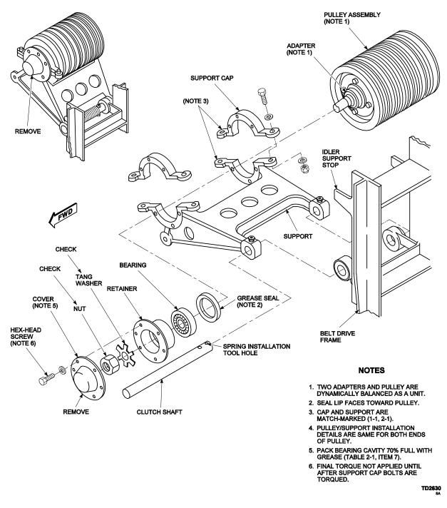
FIGURE 1. Adapter-Mounted Idler Pulley Clutch Installation (One-Piece Support)
