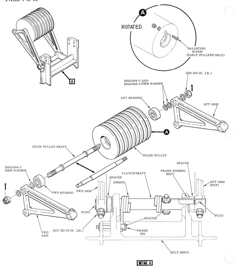
FIGURE 1. IDLER PULLEY CLUTCH ASSEMBLY (SHAFT-MOUNTED DUAL ARM SUPPORT)
