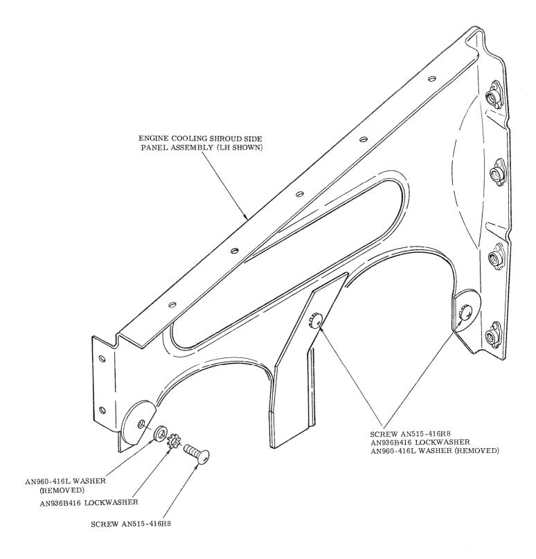
Figure 1. Engine Cooling Shroud Side Panel Assembly
