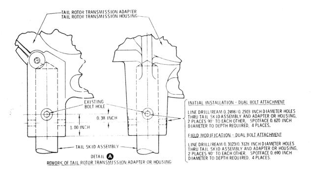
Figure 1. Field Installation and Modification - Dual Bolt Tail Skid Mounting Hardware
