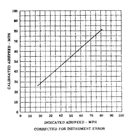
Figure 3-1. Airspeed Calibration Curve
