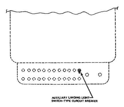
Figure 4-1. Auxiliary Landing Light Switch-Type Circuit Breaker
